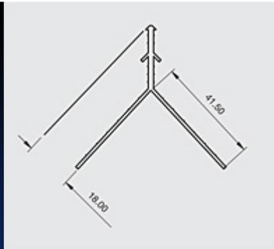
Locally manufactured from recycled plastic, Renderplas PVC corner beads / angle beads are designed for function and speed on all external and internal rendering and plastering applications. Discreet but strong, all beading gives a perfect finish to through colour render and is equally suitable for sand and cement
