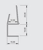
Locally manufactured from recycled plastic, Renderplas PVCu architrave shadow gap beads are designed for plasterboard to quickly and accurately form a shadow gap and provide a superior clean finish. Used at the edges of the plasterboard next to door frames, ceilings and skirting boards where the adjacent finish is hidden
