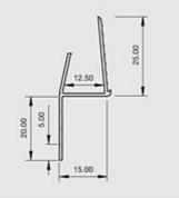
Locally manufactured from recycled plastic, Renderplas PVCu architrave shadow gap beads are designed for plasterboard to quickly and accurately form a shadow gap and provide a superior clean finish. Used at the edges of the plasterboard next to door frames, ceilings and skirting boards where the adjacent finish is designed to be seen
