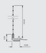
Renderplas PVC reveal beads with integrated foam vibration strip and glass fibre reinforcement mesh. Designed to protect frames and surfaces in reveals and extend the life of render and EWI systems
